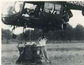
2. Carrying a pilot and three fire fighters, the HOK hovers over fire fighting equipment while ground crewman hooks it to the ship.
