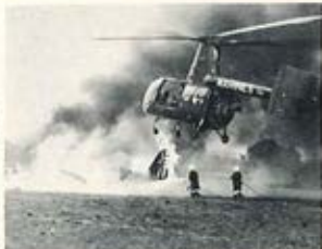
5. Hovering over the flames, the HOK uses the powerful downwash of air from its rotors to beat down the fire. Firemen go into action.
