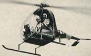
The Army H-32, powered with ram jet engines.
