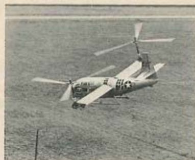
ON THE WAY —Bell XV-3 Convertiplane has made conversions up to 15 degrees forward most angle in flight without incident during the Phase I tests conducted at the Bell Aircraft plant in Texas. Evaluation flights in the helicopter configuration indicate low power requirements in forward flights up to 80 knots. Vibration level is low; autorotation checks from 500' reveal excellent power-off characteristics.
