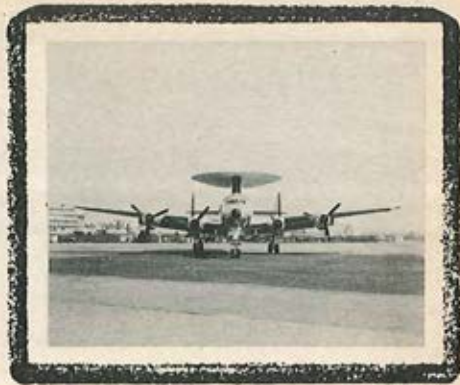
FLYING SAUCERS? Don't shoot, it's friendly! The disc-shaped saucer sitting atop a U. S. Navy WV-2 Super Constellation is a new type radome, containing radar antenna and measuring more than 30 feet across. The new piggyback pancake was scheduled for taxi-tests on the runways at Lockheed's Burbank plant, prior to later re-assembly on the plane at Edwards AFB.
